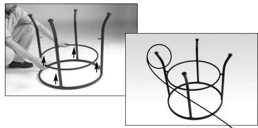
**3b.** Install four foot pads, one into each leg.
